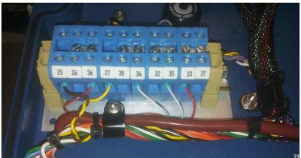
Remove wires on terminals TB2 (located in the lid, (photo above) - 34 (white), 32/35 (white), 33/37 (red) and 36 (red)
