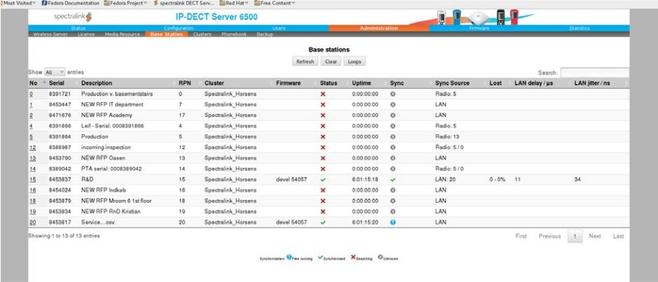
The screenshot shows the 'Base Stations' page in the Spectralink administration interface. The table lists 20 base stations with columns for No, Serial, Description, RPN, Cluster, Firmware, Status, Uptime, Sync, Sync Source, Lost, LAN delay / μs, and LAN jitter / ns. The 'Sync' column shows a blue icon for the master (entry 20) and a green icon for slaves. The 'Lost' column shows a percentage and a counter for entry 15.
