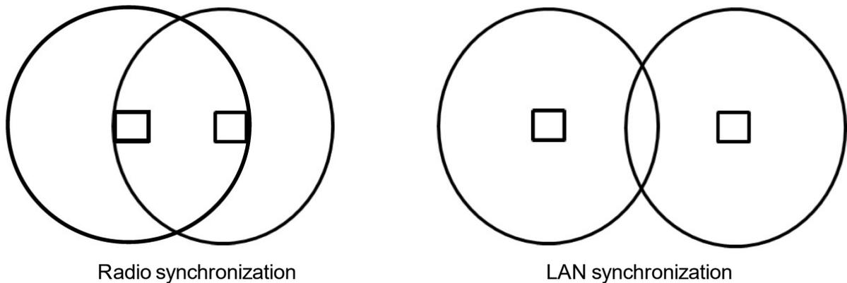
It should be noted that depending on the deployment - Synchronization via LAN and radio can be combined in the same DECT installation. Even when a base station is configured to synchronize via LAN, it transmits the signal required for synchronization via radio. Therefore, base stations synchronizing via radio can retrieve their synchronization signal from a base station synchronizing via LAN. The other way around is not possible.
