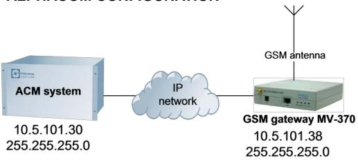
The SIP GSM Gateway must be equipped with a SIM card and registered to the GSM network as a regular mobile phone subscriber. Via the gateway, calls can be made from the AlphaCom XE to the GSM network, as well as from the GSM network in to the AlphaCom XE.
