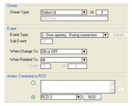
During a conversation between a door station and a telephone, the telephone operator can activate the Door Opening feature in the AlphaCom by pressing digit 6.
