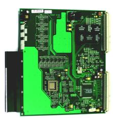
The APC Board (1009301000) is used in AlphaCom XE20 and XE26 to control the backplane board clocking. It also controls the speed of the fans.
