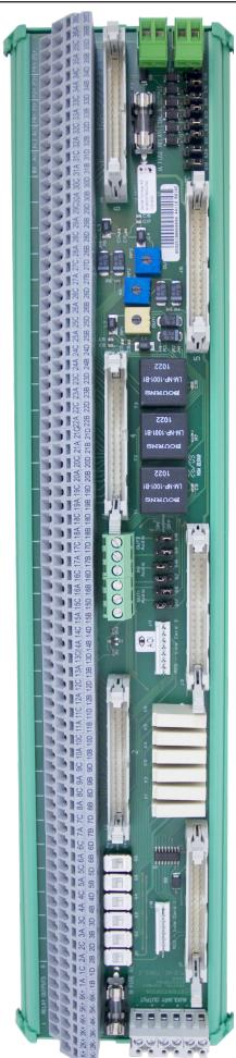
The Line Connection Module (LCM) is used for external connections for the AlphaCom XE / ACM exchanges with any mix of ASLT, ATLB and ATLB12 boards.
