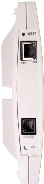
Figure 23 Faceplate showing Ethernet port
