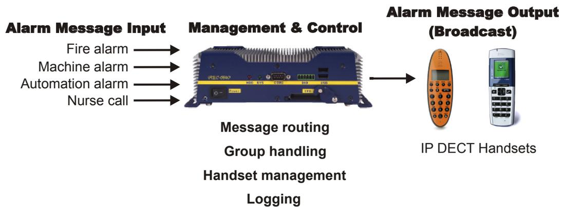
The IP DECT Alarm Server is installed and configured as part of the IP DECT 6000 System.
