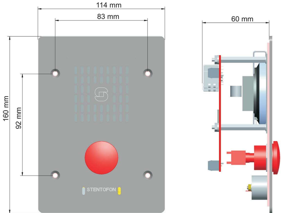
Figure 7 IP Substation (3 Gang) Dimensions
