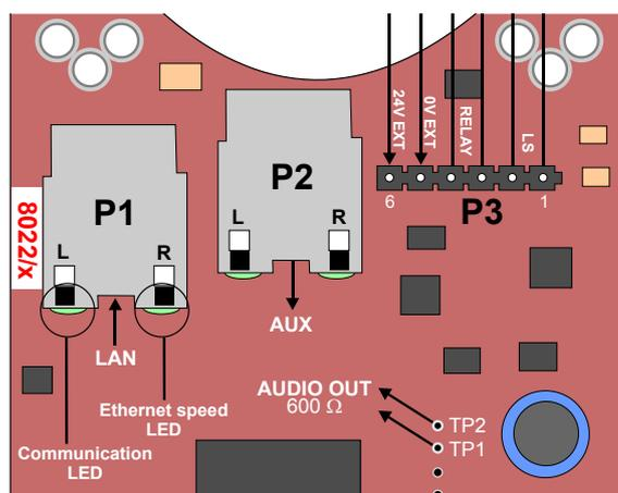
Figure 2 RJ45 Ports (P1 & P2) on PCB of IP Substation
