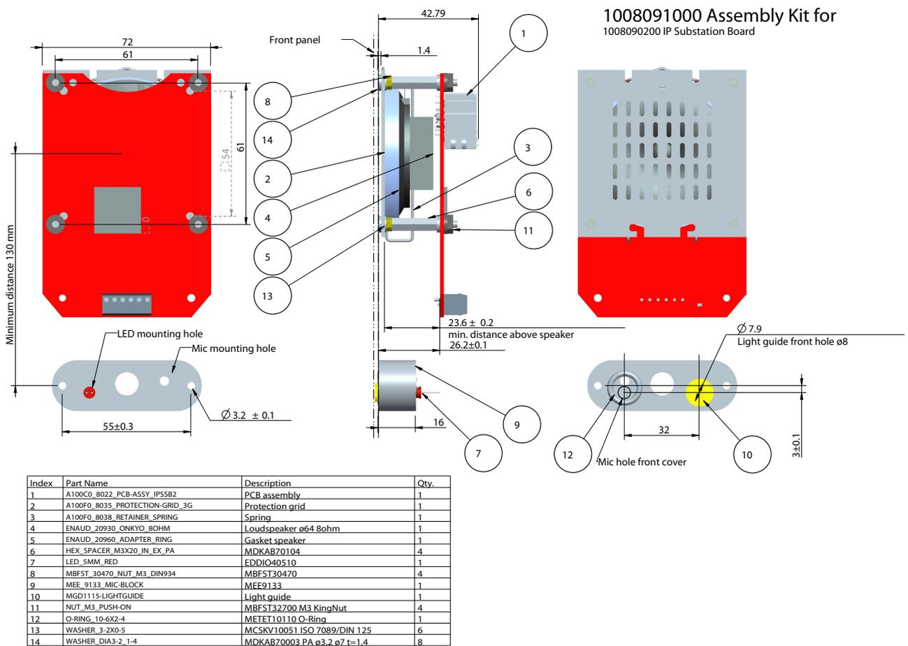
Figure 11 IP Substation Assembly Kit Mounting Dimensions
