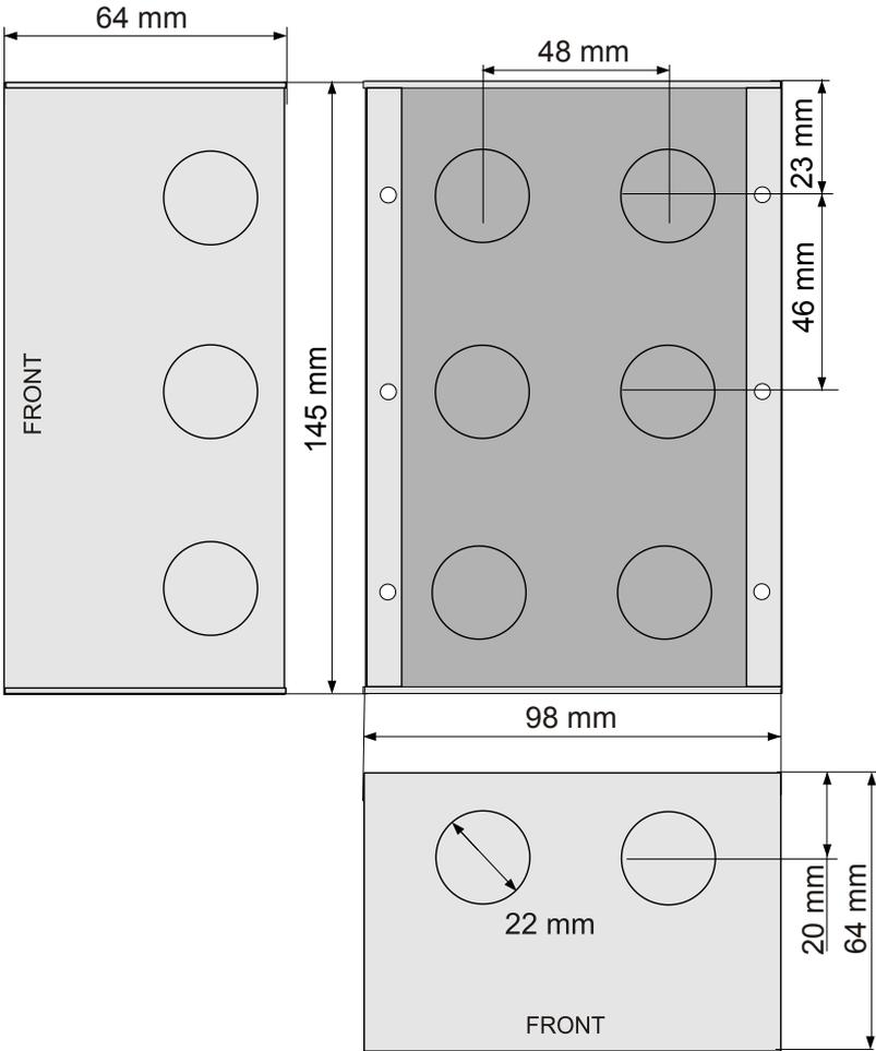
Figure 8 IP Substation - 3 Gang Backbox
