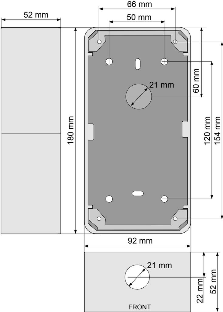
Figure 6 IP Substation - Surface Mount Backbox
