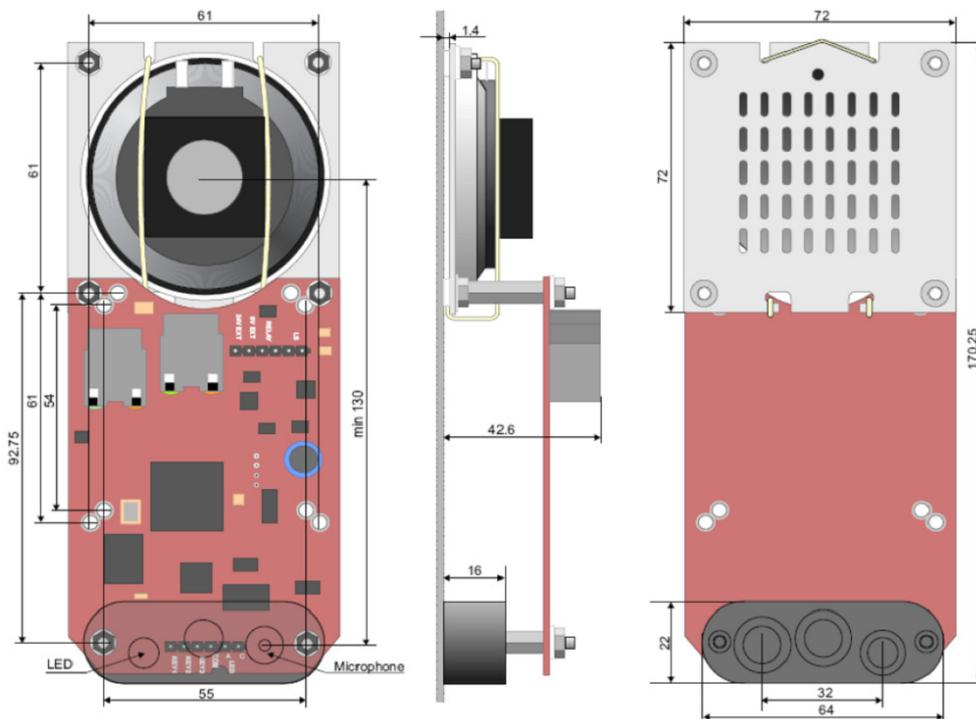
Figure 7 Substation Kit Mounting Dimensions (mm)
