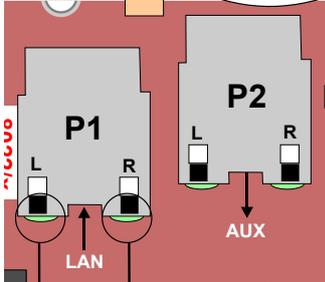
Connect both the PC and the SIP substation to a PoE switch and the LAN port (P1) on the IP intercom substation to the PC via the switch.
