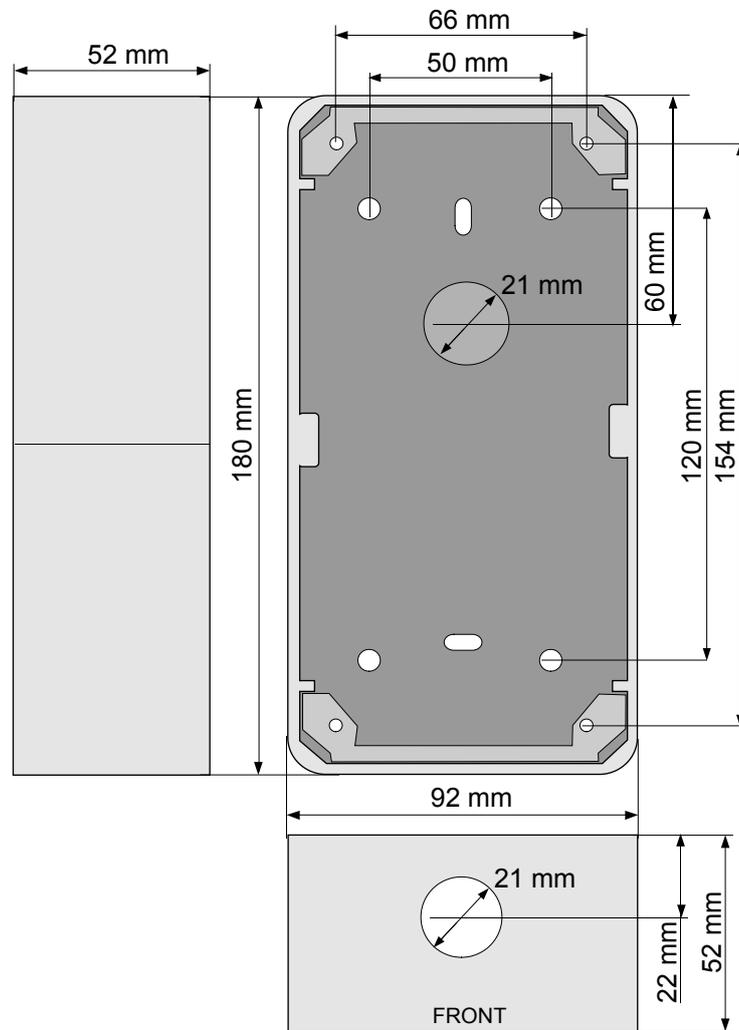
Figure 6 SIP Substation - Surface Mount Backbox
