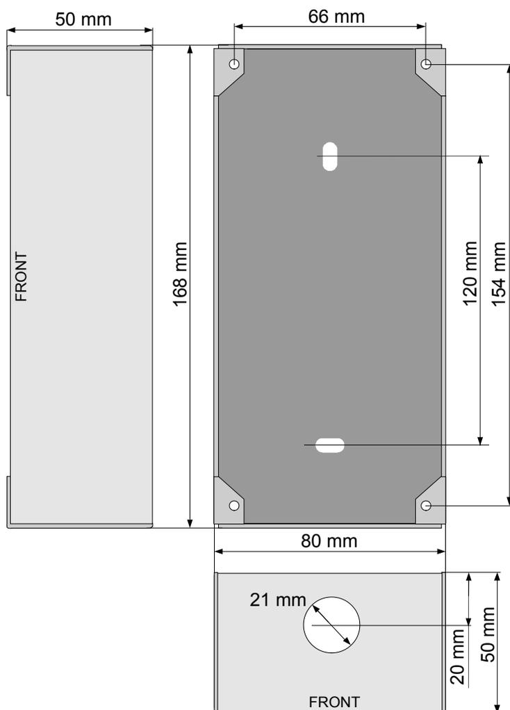
Figure 5 SIP Substation - Flush Mount Backbox
