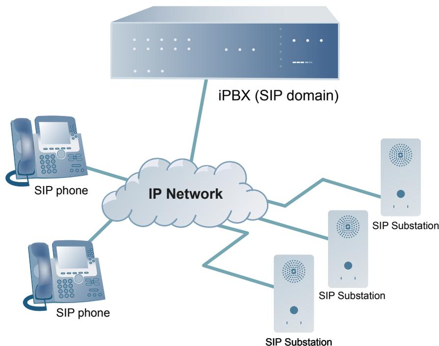
Figure 1 System Configuration
