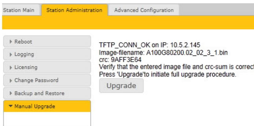
Click the **Upgrade** button to start the software upgrade procedure for the SIP substation. The upgrade procedure takes approximately 3 minutes.
