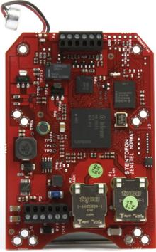
The STENTOFON SIP Substation Kit features the same electronics board (PCB) that is used in its own IP substations. It is designed to build stations to the highest specification and for use in the harshest of environments. Like all STENTOFON stations, the SIP Substation Kit features superb audio quality. This is enabled through a set of advanced technologies such as active noise filtering, acoustic echo cancellation, wide band audio codec, and high power audio outputs.
