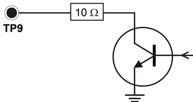
⚠ Note that the amplifier input **MUST BE AN AC COUPLED INPUT** (transformer, capacitors, etc.).
