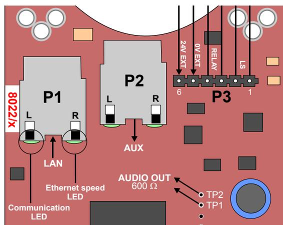
Figure 2 RJ45 Ports (P1 & P2) on PCB of SIP Substation
