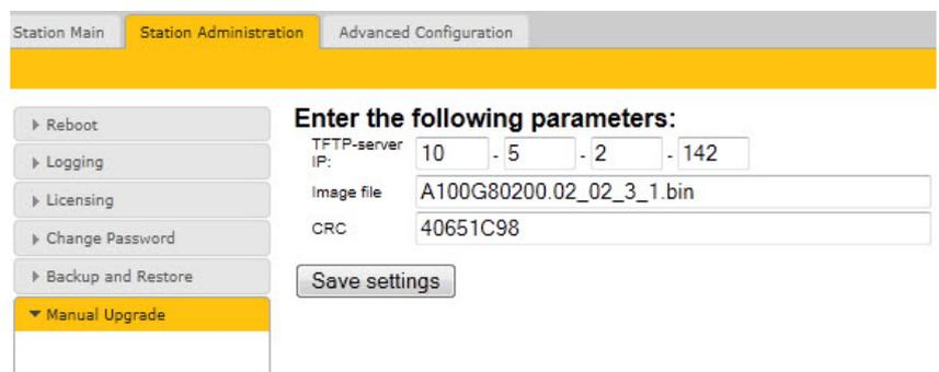
4. Enter the IP address of the **TFTP server** (your PC IP address)
