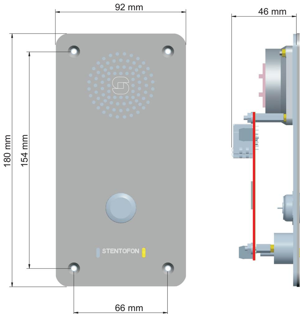
Figure 4 SIP Substation Dimensions
