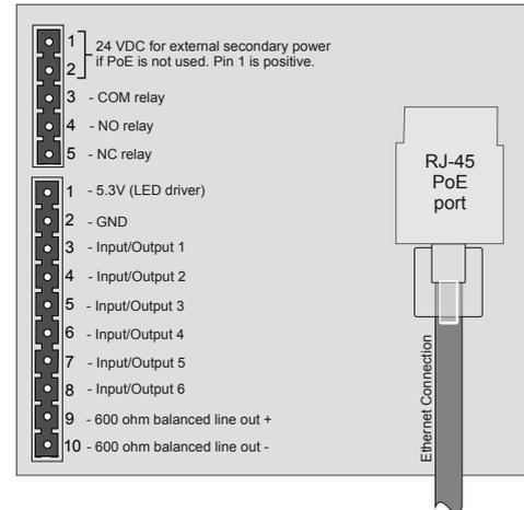
The following table is an overview of the main connectors involved when installing the Turbine IP Stations.
