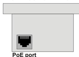
There is one RJ-45 port located on the Turbine station that is used as the PoE/LAN port.
