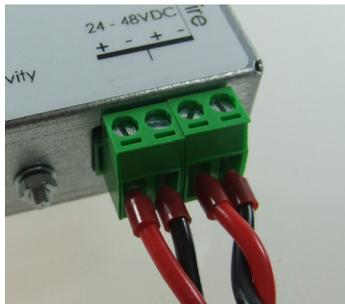
The Flowire Converter must be connected to the Flowire star configuration using twisted cabling as shown. The red wire is the positive supply voltage while the black wire is the negative supply voltage. The power supply voltage used depends on the type of devices in the star configuration.
