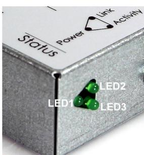
The Flowire Converter is equipped with three green LEDs. These indicate the status of the power, the connection/link to Flowire, and whether data is transmitted on Flowire or not.
