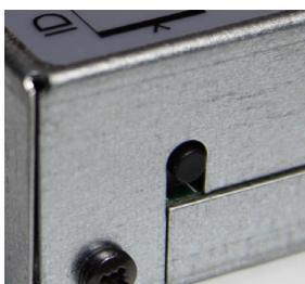
Pressing and holding this button for more than 15 seconds will reset the NMK password to the default: **HomePlugAV0123**
