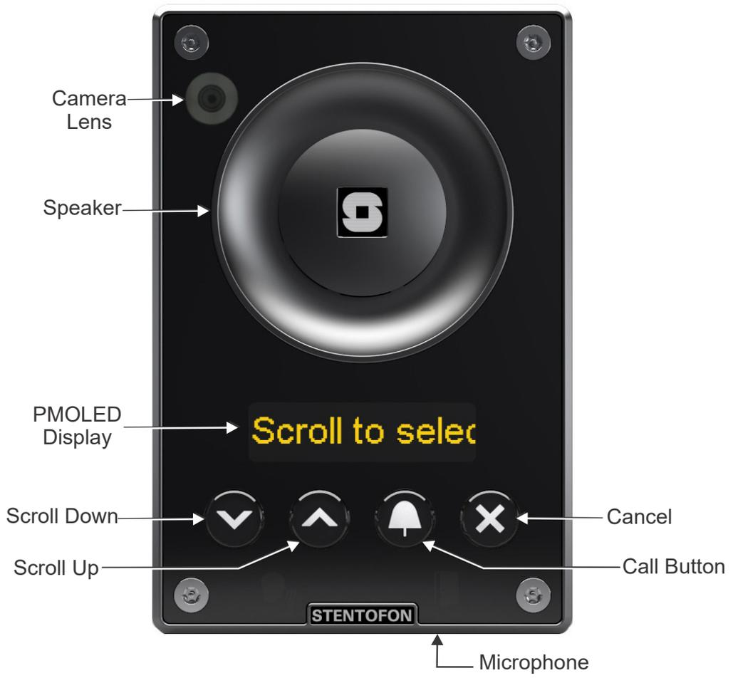
Figure 2 Turbine TCIV-6 Station Keys & Functions
