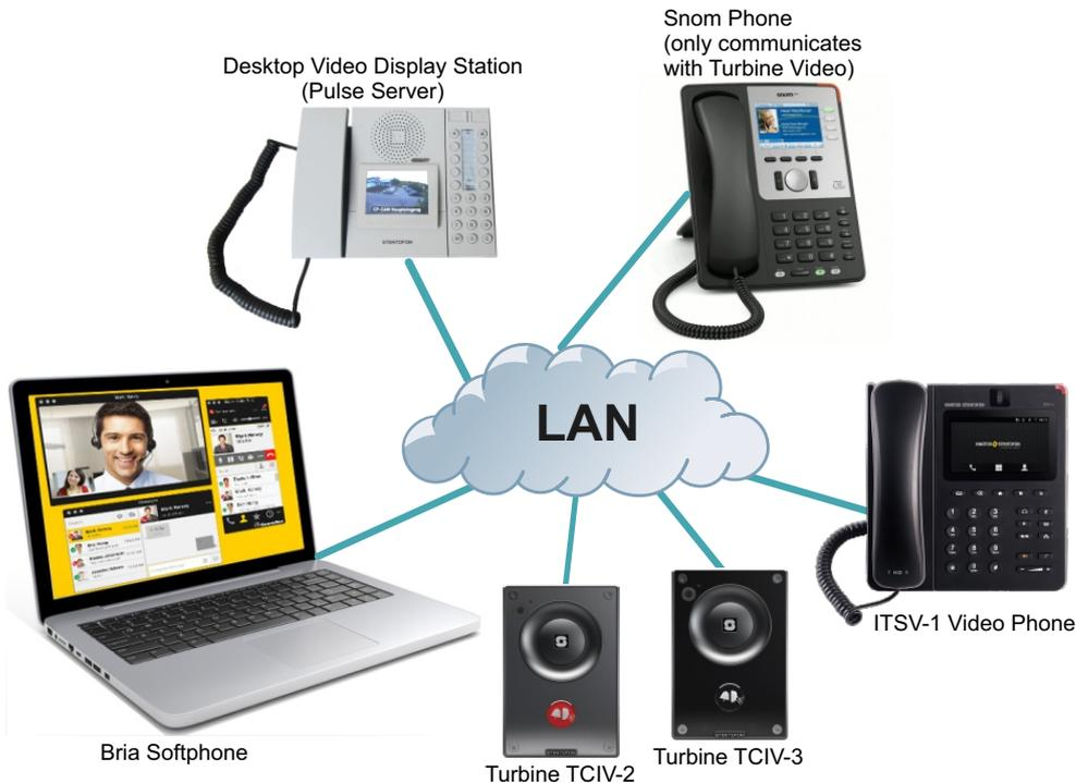
Figure 7 Pulse Video Intercom System
