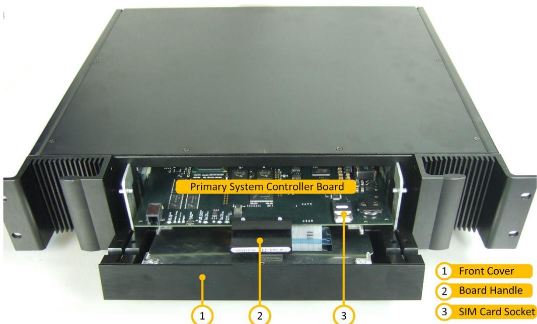
Figure 3: PSC Board in System Controller
