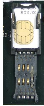
Figure 7: SIM Card in Socket
