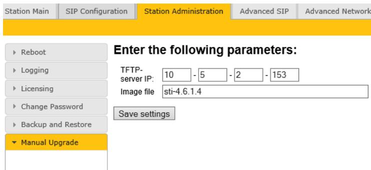
4. Enter the **IP address of the TFTP server** (your PC's IP address)
