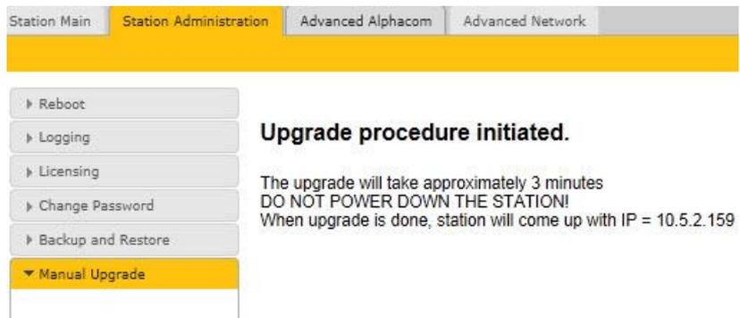
The upgrade procedure takes about 3 minutes. The process can be monitored by clicking the **Log viewer** tab in the TFTP server program.
