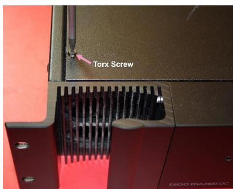
Figure 1: Removing Top Panel
