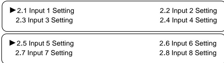
Under this interface, users can use UP or DOWN key to choose channel, and press ENTER to go to the relevant submenu for setting parameters.
