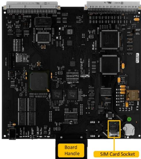
The AMC-IP processor board is used both in the AlphaCom XE audio server and the Exigo ESC1 system controller.
