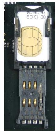
Figure 4: SIM Card in Socket
