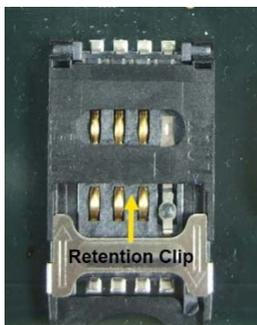
Figure 1: Retention Clip Closed
