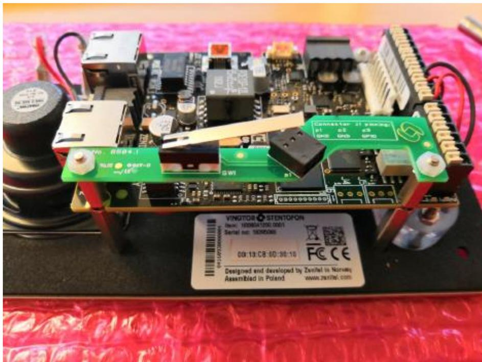
**4 Remove the button GND wire from the TKIE board**
