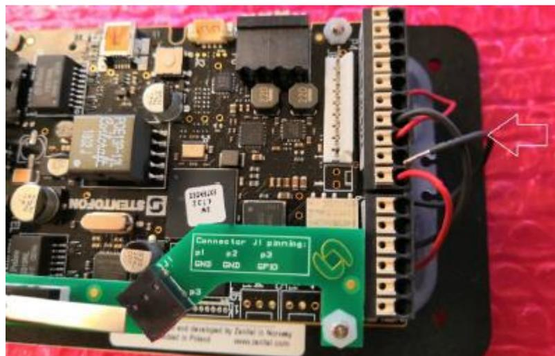
**5 Insert the button GND wire into the connector on the tamper switch as shown**
