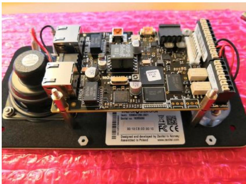
**3 Mount the tamper switch on top of the spacers and secure with the nylon nuts**
