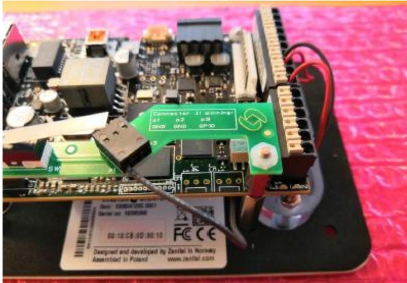
**6 Use the supplied wires to connect GND and GPIO as shown**
