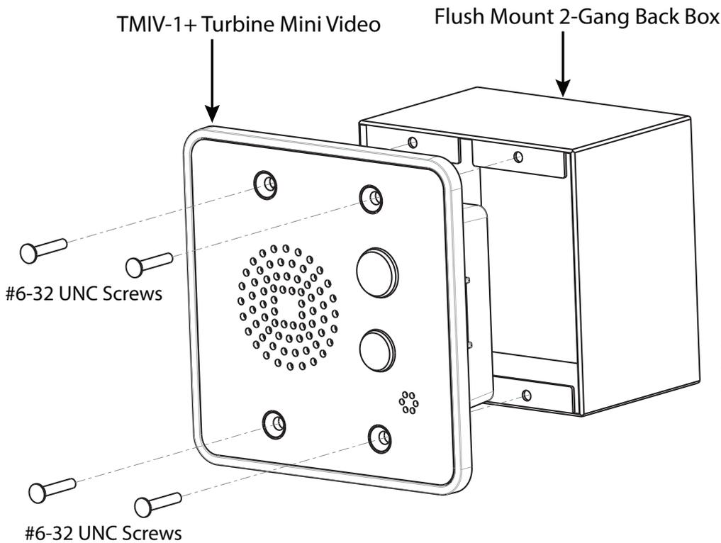
To attain the rated ingress protection of IP44, flush mounting of TMIV-1+ must only be done on a surface that is completely planar, smooth, and clean. Any surface irregularities must not exceed 0.5 mm. If this is not achievable in a reliable manner, appropriate sealant or filler should be applied to seal the gap between the station and the wall. Optionally, the on-wall back box TA-32 could be used.
