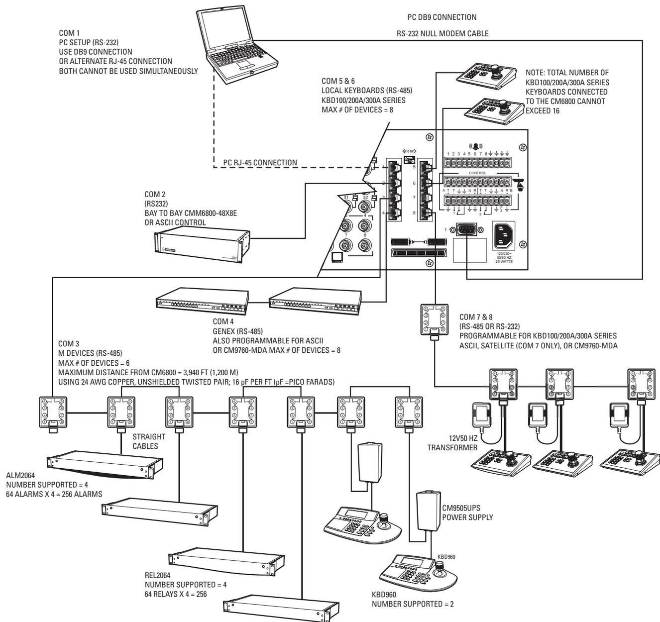
**Figure 13. CM6800E Communication Port Connections and Options**
