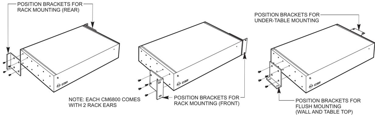
**Figure 4.** Installing Rack Ears
