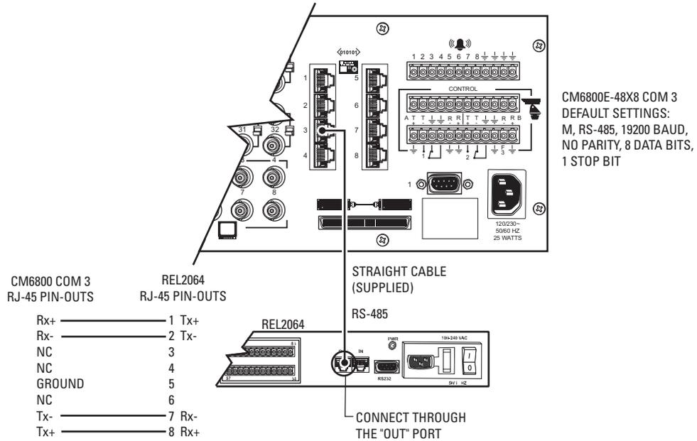
**Figure 20.** Connecting a Single REL2064 Relay Interface Unit
