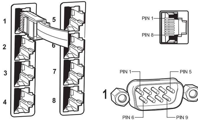
**Figure 12.** Communication Port Inputs
