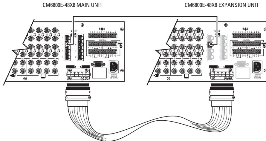
**Figure 28.** Data and Video Connections Between CM6800E-48X8 Units
