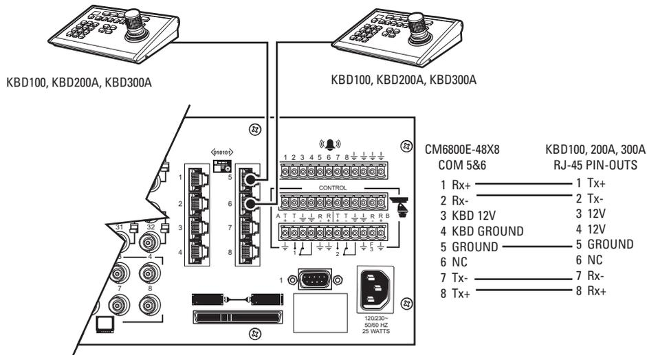
Figure 15. Data Cables Plugged into COM 5 and 6
