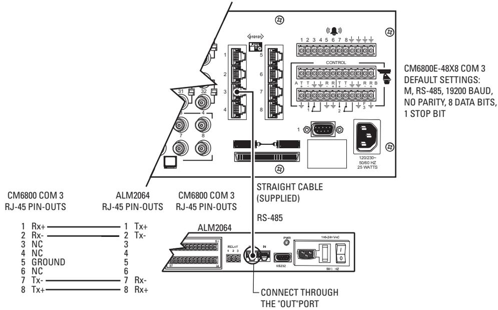
Figure 19. Connecting a Single ALM2064 Alarm Interface Unit
