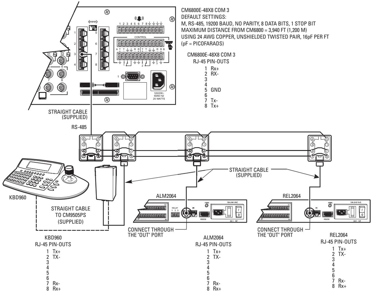
Figure 22. Connecting Multiple M Devices – Remote Connection
