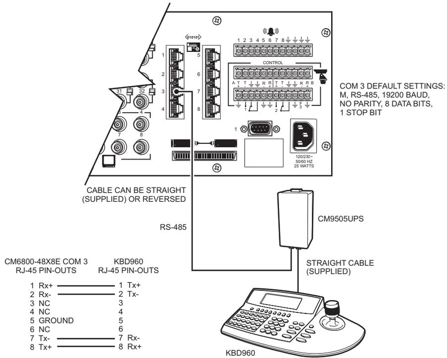
**Figure 18.** Connecting a KBD960/KBR960 to the CM6800E
