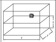
Category W-x-y (Wall mounted): Wall mounted, where x is the maximum mounting height from the floor and y is the maximum length of the sides of the square floor area covered by the VAD.
