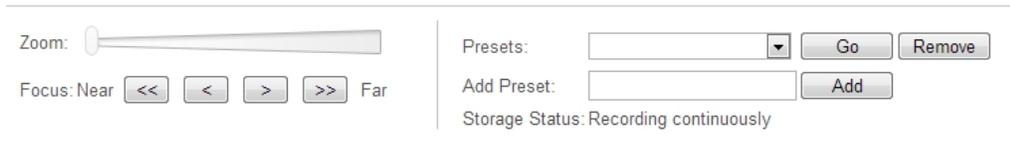
1. On the Live View page, use the Zoom and Focus controls to focus the camera on a specific point in the video image.
