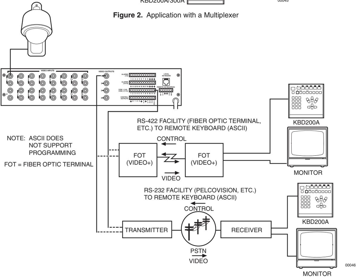
Figure 3. Applications with Remote Keyboards (ASCII, KBD200A Only)
