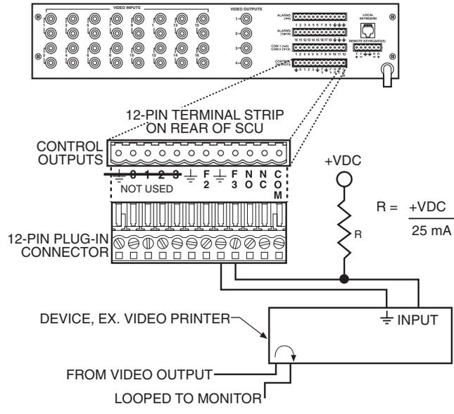
+VDC = VOLTAGE OF THE EXTERNAL POWER SOURCE
